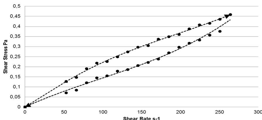
Figure 2. Example to thixotropic hysteresis curve for unripe grape juice; for 20% SSC, at 40°C
