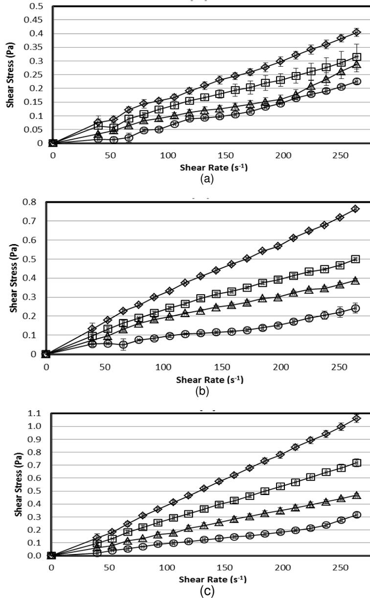
Figure 1. Rheograms for shear stress versus shear rates plots of unripe grape juice concentrates at various temperatures 10°C ( $\diamond$ ), 25°C ( $\square$ ), 40°C ( $\Delta$ ), 80°C ( $\circ$ ) for concentrations of (a) 4.6 % SSC, (b) 15 %SSC, and (c) 25 % SSC.
